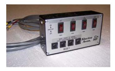
The switchbox (12 volt DC), consists pf illuminating rocker switches. Light in switch indicates when rows are shut off. Circuit breakers protect the solenoids which apply secondary release wheels.
